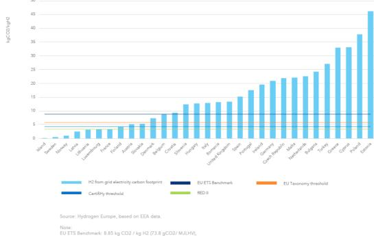
Figure 1: Carbon intensity of hydrogen produced from grid electricity (without extra measures), compared to selected benchmarks.
