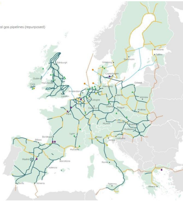
Figure 3: European Hydrogen Backbone 2040, about 40,000 km hydrogen pipelines, 70% retrofitted gas pipelines and 30% new constructed hydrogen pipelines (GasforClimate, 2021)
