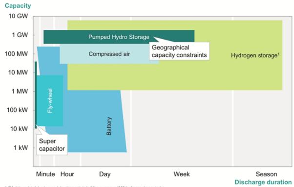
1 IEA data updated due to recent developments in building numerous 1MW hydrogen storage tanks Source: IEA Energy Technology Roadmap Hydrogen and Fuel Cells, JRC Scientific and Policy Report 2013
